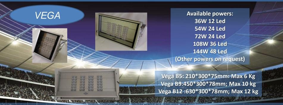
New generation LED projectors, innovative design suitable great areas such as for sport and leisure facilities and also tunnels. Die-casted gray aluminium body and upper shell, equipped with cooling fins for a optimal dissipation and extension of the LED's useful life. High transparency (higher than 95%) 4mm thick tempered glass diffuser. The silicone gaskets ensure maximum sealing against weather conditions.
