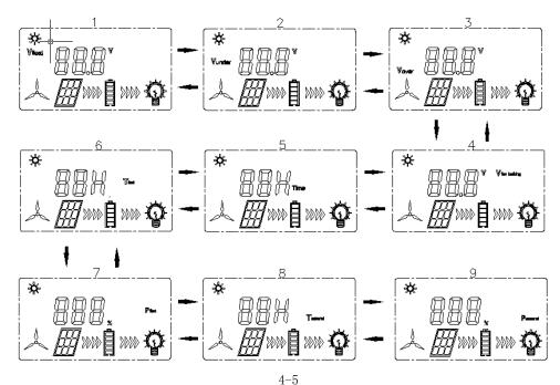
The controller can be set to Float charging pressure point "VFloat",under-voltage point "Vunder", over-voltage point"Vover",fan unloading point "Vfan\_breaking",the operation method is the same as the first item.
